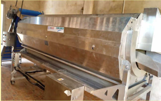
5 tons per hour Stainless Steel Fresh Ginger washer equipped with Food Grade intake and Delivery Elevators
