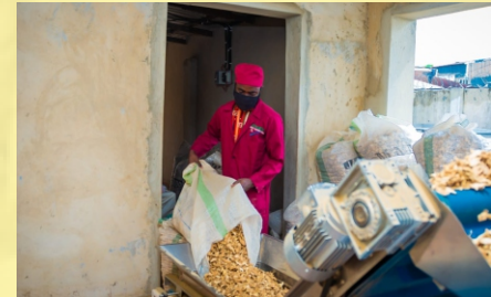
Removal of Metallic Contaminants from GACON Ltd's Dried Slip Ginger using Electromagnets
